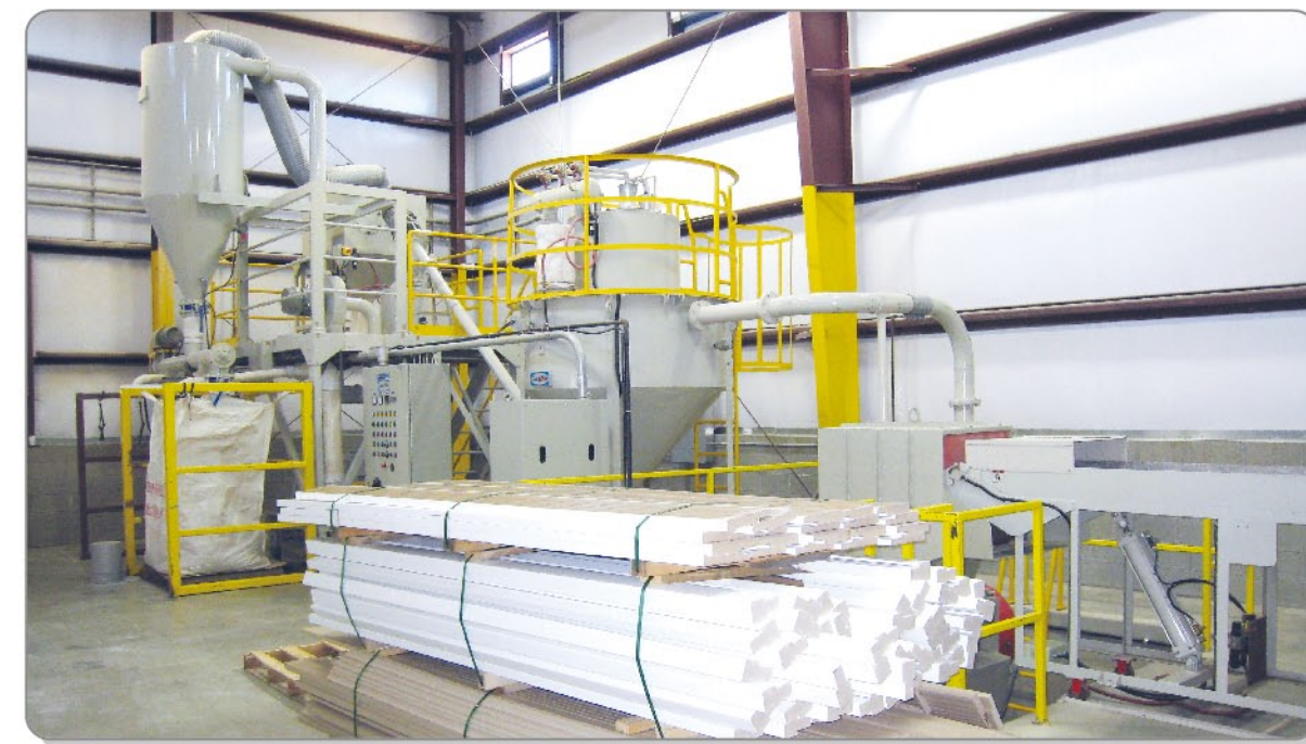
▲ PVC+木粉料從粉碎到磨粉一貫作業流程 PROCESSING OF PVC & WOOD FROM CRUSHING TO PULVERIZING
